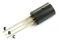
A transistor is kind of like an electronic dimmer switch.
