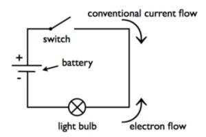
In this schematic, the battery, switch and LED are connected so the LED will light up when the switch is turned on. Just spend a minute looking at this schematic until it makes sense to you. Then try drawing one yourself of another circuit you've built.
