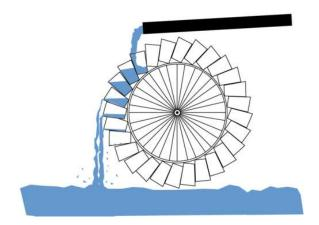
The pump is like a battery, the hoses like wires, and the water wheel is like a light bulb, motor, or anything else that uses electricity. If we haven't decided what to hook up there yet, we sometimes just call it a *device*. Now, as long as the pump is going, the water wheel turns. What would happen if you pinched the hose? The flow of water would stop and the water wheel would stop. This is what a switch does in a circuit—it stops the flow of electricity.
