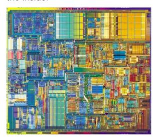
It's a square piece of crystallized silicon containing millions of tiny transistors connected by *very* tiny wires.
