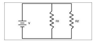
There's an equation for calculating it (called the parallel resistance formula). But the general idea is that half the current goes through each one. So, if you connected two 100 Ohm resistors in parallel, you would end up with the equivalent of a 50-Ohm resistor.
