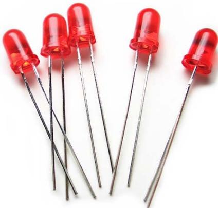
Sometimes, we put LED's in shapes to make numbers or letters on digital displays, like on a digital clock. If your clock lights up in color, it's probably an LED display (black on grey are LCD displays, not LED).
