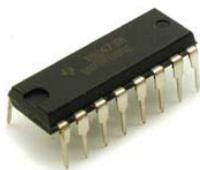
with wires coming out of it. Most chips are just 5mm to 20 mm long and wide. They come in different shapes, and have different numbers of wires (called "leads") coming out of them.
