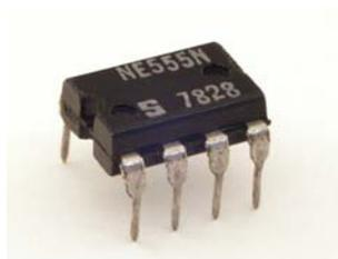
with wires coming out of it. Most chips are just 5mm to 20 mm long and wide. They come in different
